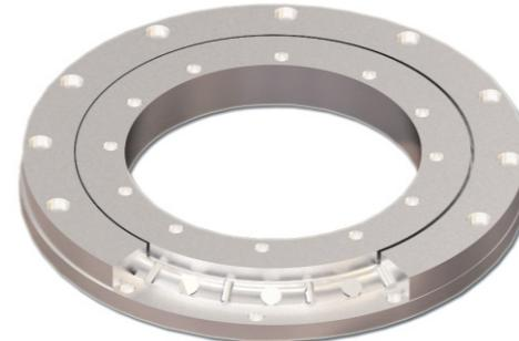
Due to the X arrangement of the cylindrical rollers, these bearings can support axial forces from both directions as well as radial forces, tilting moment loads and any combination of loads by means of a single bearing position. As result, designs involving two bearing positions can be reduced to a single bearing position.
